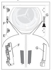
**Note regarding contact protection:** The machine is only secure for operations again once all plastic parts have been inserted.
